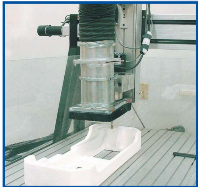
The CNC Machine Center produces exact product prototypes
